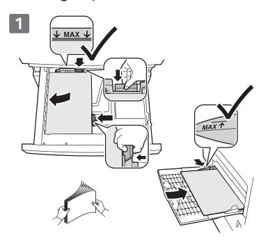
For best results, fan the edges of the paper. Adjust guides to fit the paper size. Do not load paper above the maximum fill line.
