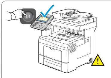
To prevent a printer malfunction or damage to the internal hard drive, touch the Power button on the control panel and respond to the prompt. For full Power Down, after 10 seconds the touch screen goes dark and the Power Saver button flashes. When all of the control panel lights are off, turn off the power switch.
