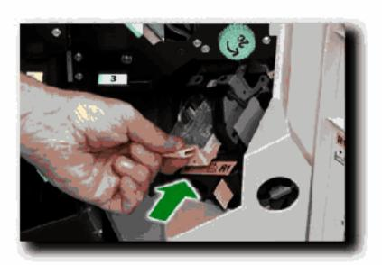
Unpack and install the new staple cartridge in the finisher. The staple cartridge clicks into place. Rotate the stapling unit to its home position, and close the Finisher Front Door.
