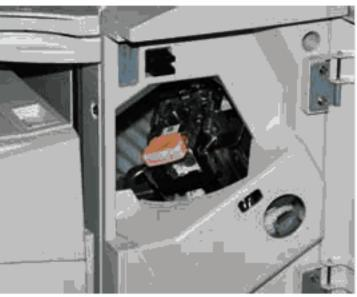
This procedure shows you how to remove an empty staple cartridge from the Office Finisher and replace it with a new staple cartridge.
