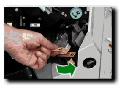
To gain access to the staple cartridge, open the Finisher Front Door and rotate the stapling unit counter-clockwise.
