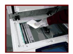
Use a lint-free cloth, lightly dampened with Xerox Anti-Static or General Cleaning Fluid or another suitable non-abrasive glass cleaner, to clean the glass area.
