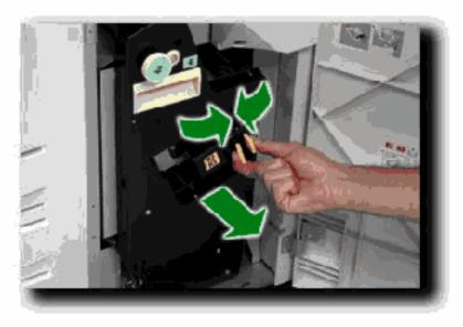
To gain access to the Booklet Maker staple cartridges, open the Finisher Front Door, and pinch the two Booklet Maker Access handles together. Pull out the Booklet Maker stapling unit.
