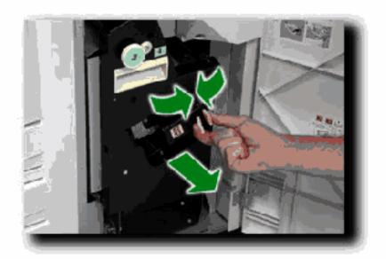
To gain access to the Booklet Maker staple cartridges, open the Finisher Front Door, and pinch the two Booklet Maker Access handles together. Pull out the Booklet Maker stapling unit.
