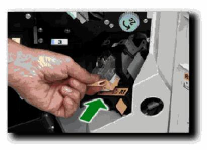
Unpack and install the new staple cartridge in the finisher. The staple cartridge clicks into place. Rotate the stapling unit to its home position, and close the Finisher Front Door.
