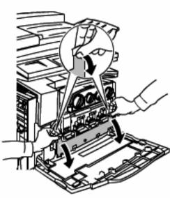
3. Open the Waste Toner Container door by grasping the two door tabs and pull it down.
