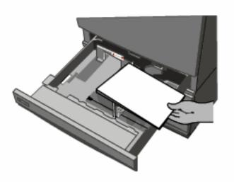
Register the stack of paper against the front left-hand corner of the tray. Paper must not be loaded above the maximum fill line.
