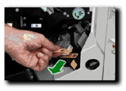
Pull up on the staple cartridge handle and remove the used staple cartridge. Dispose of the staple cartridge according to the instructions contained in the new staple cartridge box.
