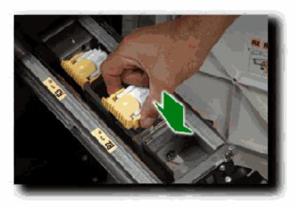
Unpack and install the new staple cartridge. The staple cartridge clicks into place. Return the Booklet Maker stapling unit to its home position, and close the Finisher Front Door.
