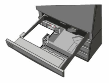
Trays 1 and 2 can take 520 sheets of 20lb/80gsm media, in sizes from 5.5"x8.5"/A5 to 11"x17"/A3.
