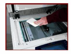
Use a lint-free cloth, lightly dampened with Xerox Anti-Static or General Cleaning Fluid or another suitable non-abrasive glass cleaner, to clean the glass area.
