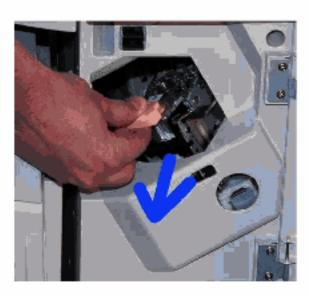
Pull up on the staple cartridge handle and remove the used staple cartridge.
