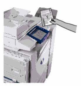
To ensure optimum print quality at all times regularly clean the glass areas of your machine. This helps avoid output with streaks, smears and other marks that transfer from the glass area when scanning documents.
