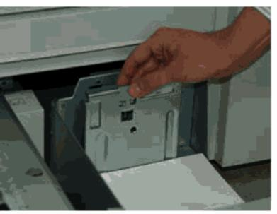
Open the appropriate Tray and move the rear guide to just touch the rear edge of the paper stack.
