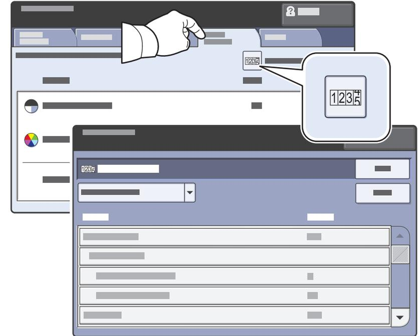
EN In the Machine Status menu, touch the Billing Information tab for basic impression counts. Touch the Usage Counters button for detailed usage counts.
