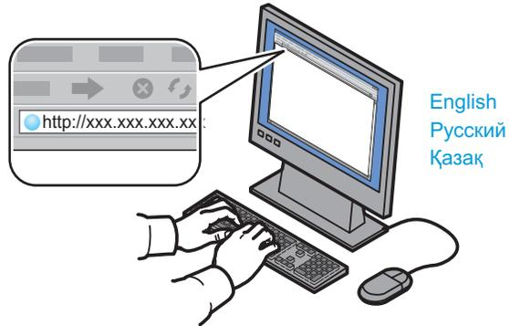
**EN** CentreWare Internet Services enables you to access printer configuration, security settings and diagnostic functions, and to manage address books and scanning over a TCP/IP network. To connect, type the printer's IP address in your computer's Web browser. The IP address is available on the Configuration Report information page.
