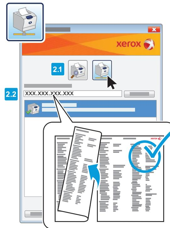
EN If your printer is not discovered, click the network printer icon, enter your printer's IP address, then continue setup. The IP address is available on the Configuration Report. To print a Configuration Report, see page 7.
