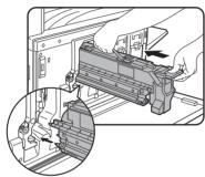
Align the insert holes as shown and then push the cartridge in.
