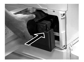
After installing the Toner Cartridge, pull the Charger Wire Cleaning Lever out of the Drum Cartridge until it stops and then push it back in again several times. This process cleans the charger wire.
