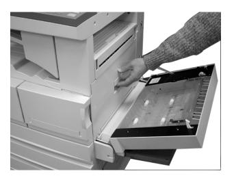
Remove the cleaning tool from its storage space on the machine.
