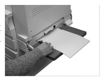
**NOTE:** The Bypass tray is extendable to accommodate short edge feed sheets or larger paper sizes.
