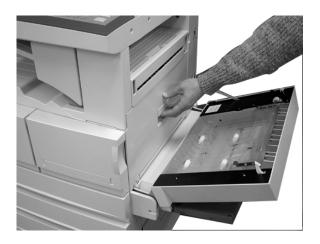
Remove the Toner Cartridge using the instructions "Replacing the Toner Cartridge" on page 5-9.
