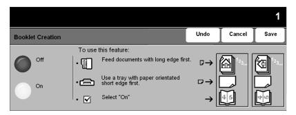
Use this feature to create multipage booklets from a sequential set of either singlesided or double-sided originals. The machine will reduce and correctly position each image to fit on the required page. When the page is folded a booklet will be created.
