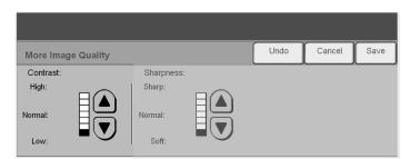
Use this feature to enhance the quality of the output based on the type of original being scanned.
