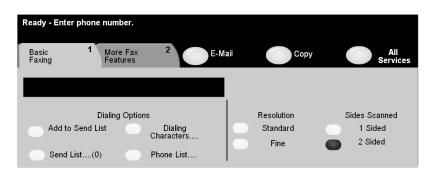
The *Basic Faxing* tab is the default screen for the Fax function. Use this tab to enter the recipient telephone number and to select the standard features for a fax job.
