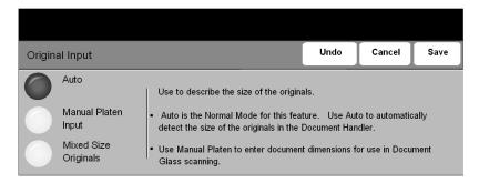
Use this option to program the size of the originals being scanned or enable the machine to recognize the size of the originals.
