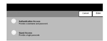
Authentication is a useful network security management tool - limiting, restricting and monitoring access to the network via the machine. Authentication can be set up by the System Administrator to restrict access to the features within Scan to E-mail, Network Scanning and Internet Fax. Once enabled, it will apply to all three services.
