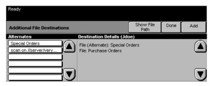
Use this feature to add file destinations to any template. A maximum of 5 file destinations can be added to a template. If the selected template contains 1 destination you can add an additional 4 destinations using this feature, however if the selected template contains 5 destinations the *Add File Destination* button is not available.
