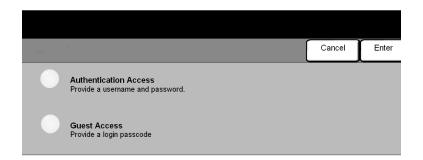
Authentication is a useful network security management tool - limiting, restricting and monitoring access to the network via the machine. Authentication can be set up by the System Administrator to restrict access to the features within Scan to E-mail, Network Scanning and Internet Faxing. Once enabled, it will apply to all three services.
