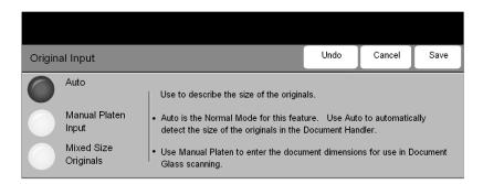
Use this option to program the size of the originals being scanned or program the machine to determine the size of the originals automatically.
