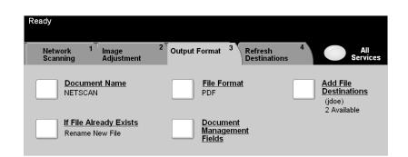
Use the features available to temporarily change the format of the scanned image file at the destination server.
