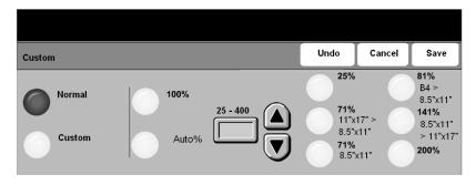
The *Reduce / Enlarge* option provides a variety of reduction and enlargement options. Originals placed on the Document Glass or sent to the machine electronically can be reduced or enlarged between 25% to 400%. Originals fed through the Document Handler can be reduced or enlarged between 25% to 200%. The preset Reduce/Enlarge options that appear on the *Copy* tab can be set in Tools mode.
