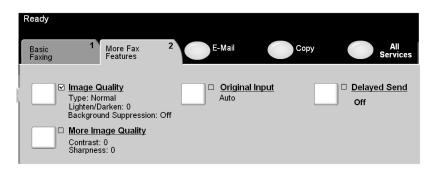
The *More Fax Features* tab provides fax features used for adjusting the appearance of the faxed output.
