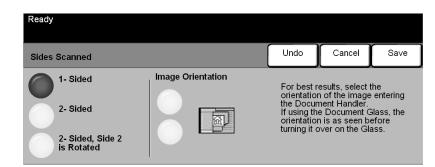
This is used to specify whether the originals are single-sided or double-sided. For 2-sided originals the orientation can also be programmed.
