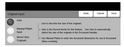
Use this option to program the size of the originals being scanned or enable the machine to recognize the size of the originals automatically.
