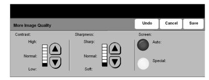
Use these features to enhance the copy quality of the output based on the quality of the original being scanned.
