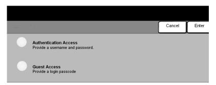
Authentication is a useful network security management tool - limiting, restricting and monitoring access to the network via the machine. Authentication can be set up by the System Administrator to restrict access to the features within Scan to E-mail, Network Scanning and Internet Fax. Once enabled, it will apply to all three services.
