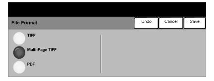
Use this feature to temporarily change the file type of the scanned image file at the destination server. The default setting is the same as the value entered in the selected template.
