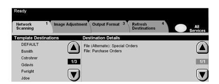
Access to the *Network Scanning* features is gained using the *Features* button on the control panel.
