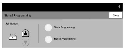
Use this feature to program up to 10 commonly used programming sequences. For example, combinations of selections such as *Edge Erase* and *Bound Originals*.
