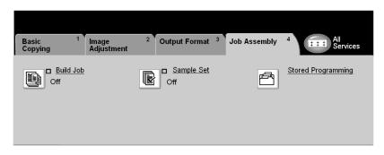
The *Job Assembly* tab is used to combine multiple documents into a single job, produce a sample set of a job or for storing the programming of up to 1000 images.
