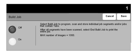
Use this feature to build a job that requires different settings for each page. For example, if a set of documents consists of some pages with text and some with photos, the appropriate setting for each original can be applied and the job can still be completed as a single job.
