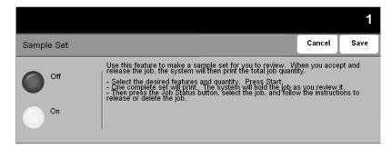
This feature is used to review the output to ensure that it is exactly what is required prior to printing a large quantity.
