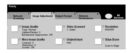
The *Image Adjustment* tab is used to progam features relating to the scanned images.
