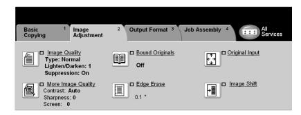
The *Image Adjustment* tab provides copy features used for adjusting the appearance of the copy output.
