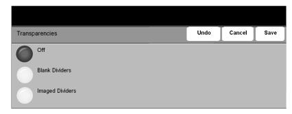
This feature allows the creation of a single set of transparencies with dividers. When dividers are selected a transparency set will always be single-sided on transparency stock with no stapling.
