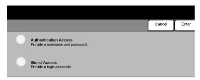
Authentication is a useful network security management tool - limiting, restricting and monitoring access to the network via the machine. Authentication can be set up by the System Administrator to restrict access to the features within Scan to E-mail, Network Scanning and Internet Faxing. Once enabled, it will apply to all three services.
