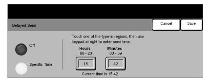
Use *Delayed Send* to specify a time, within the next 24 hours, at which to send a fax. This feature can be used to transmit faxes during off-peak hours or is useful when sending to another country or time zone. The time to send is added to the job information sent to the fax server with the scanned image. The Third Party Fax Server retains the fax for sending at the specified time.
