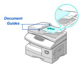
① Up to 40 sheets of 80 g/m² (20lb bond) paper can be loaded. Weight ranges from 45 - 105 g/m² (12.5 - 28lb). Sizes range from B5 to Legal (7" x 10" to 8.5" x 14"). Refer to "Scanner and Copier Specifications" on page 11-5 for full Document Feeder specifications.
