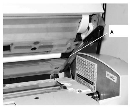
A: Calibration Roll Drive Gear
