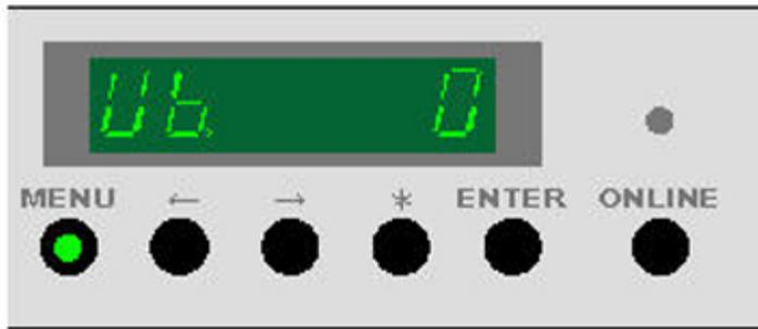
1. With the printer in the Standby (idle) condition, press the **Menu** Key 11 times to enter Mode b.
