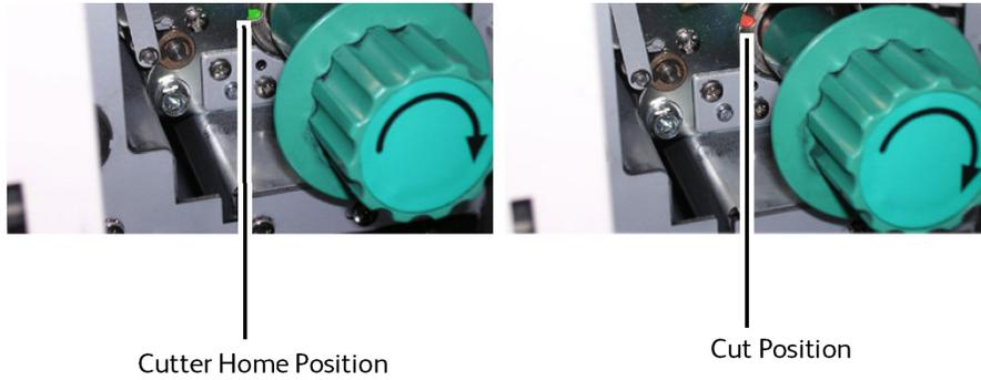
8. Return the Cutter to the home position by rotating the Cutter Knob until green is seen inside of the notch. Green indicates the home position.
