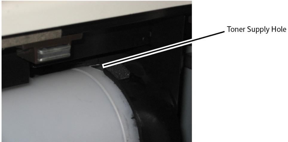
3. Pull down on the left end of the Toner Cartridge Latch and remove the cartridge by grasping the left end.
