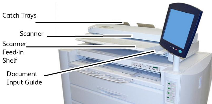
2. Evenly and gently insert the lead edge of the original into the Scanner.
