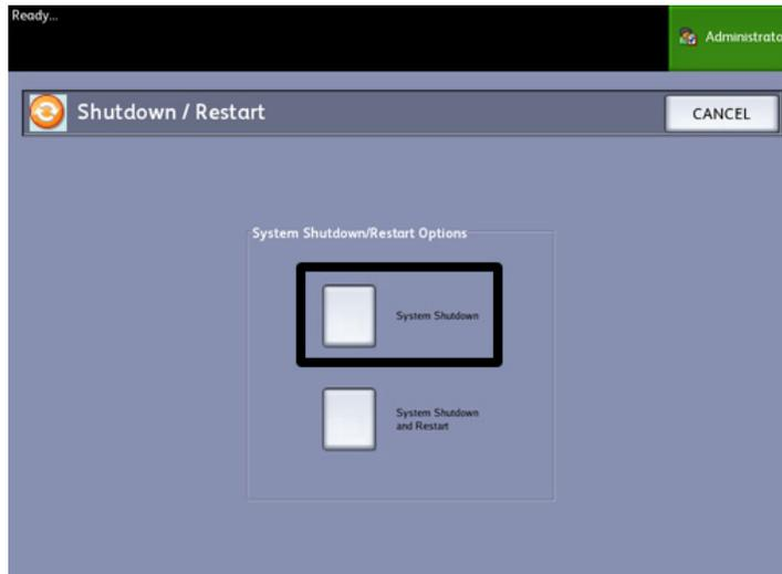
The Controller will completely shut down within 30 seconds from the moment the Printer shuts down. The Controller's Power Button Indicator Light will extinguish when the Controller shuts down.
