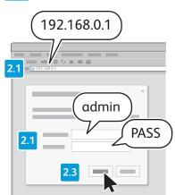
To access the web interface of the Wireless Print Solutions Adapter, open a browser. In the URL field, enter the default IP address of 192.168.0.1, then press **Enter** or **Go**. Log in to the Web interface.
