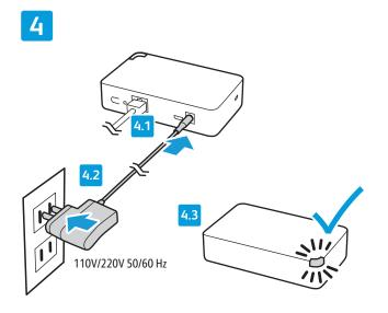
Plug in the power adapter to a wall outlet (110 V/220 V AC) or a power strip. Wait until the Status LED flashes amber.
