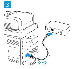
Plug the Ethernet cable into your printer and the Wireless Print Solutions Adapter.
