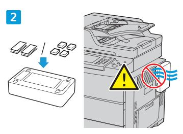
Apply the included rubber feet or hook-and-loop strips to the base of the unit. If you are attaching the device to the printer, ensure that you do not block vents or access doors.
