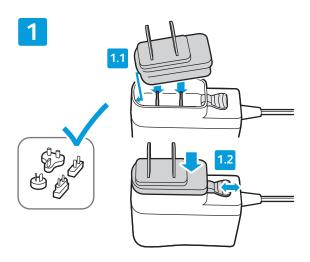
Select and install one of the AC plug adapters on the 5 VDC Power Supply. Ensure that the adapter snaps securely and fully into the base.
