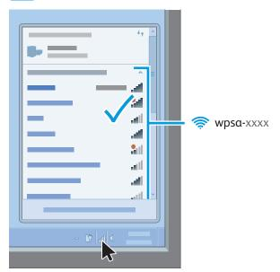
On your computer or mobile device, navigate to your list of available wireless networks. Select the available network that appears as **wpsa-xxxx** where xxxx is the last four characters of the MAC address of your adapter (not the Wireless MAC address). You can find the MAC address on the label that is located on the bottom of your adapter.
