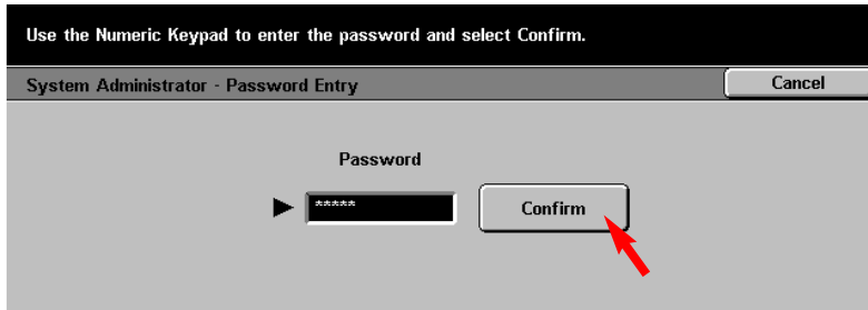
Fig. 1-2 Enter the System Administrator Password from the Numeric Keypad and then press Confirm . See Machine Administrator User Guide for default password.
