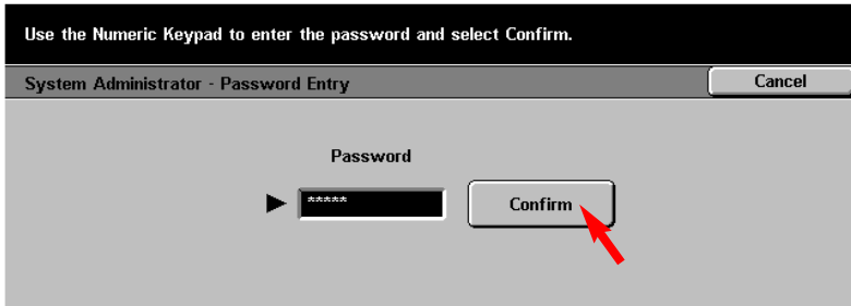
Fig. 2 Enter the System Administrator Password from the Numeric Keypad and then press Confirm . (See Machine Administrator User Guide for default password.)
