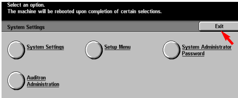
Fig. 1-12 Select Exit on the Systems Settings screen, the machine will reboot. The reboot will take approximately 5 minutes.
