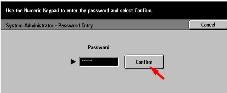
Fig. 1-2 Enter System Administrator Password using the Numeric Keypad and then press Confirm . (See Machine Administrator User Guide for default password.)
