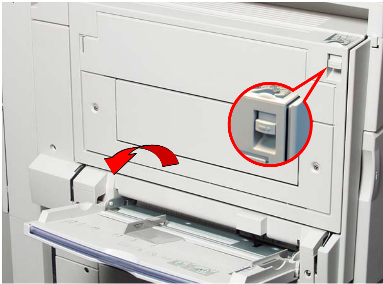
Fig. 1 Top left cover Gently open the top left cover while lifting up the release lever.
