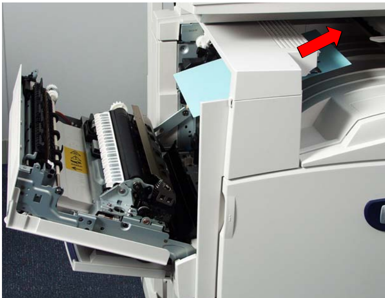
Fig. 2 If the edge of the jammed paper can be reached at the output tray, pull the jammed paper in the direction of the feed-out area.
