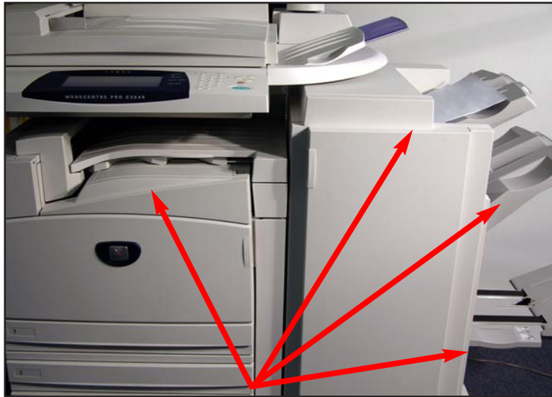
Fig. 2-9 Depending on the machine configuration and features selection the job will be delivered to one of the output trays available.
