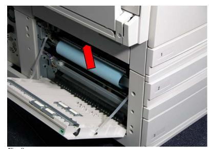
Fig. 8 **Bottom left cover**Remove the jammed paper.
