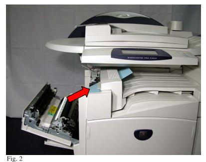
If the edge of the jammed paper can be reached at the output tray, pull the jammed paper in the direction of the feed-out area.
