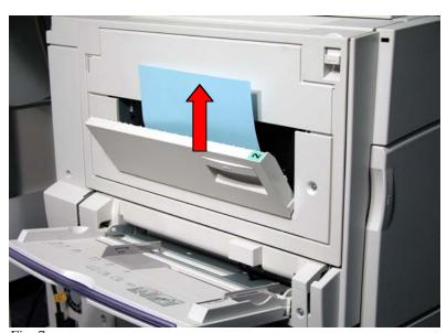
Fig. 7 **Duplex Module Cover**Remove the jammed paper.
