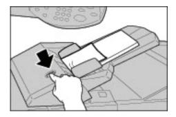
**2.** Open the cover 1e and then remove the jammed paper and all paper loaded in the Post-Process Inserter.
