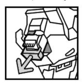
**4.** Push the positions indicated by arrows to remove the staple case from the cartridge.
