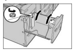
**4.** Attach the guides according to the hole of the paper size to change, and tighten the screws.
