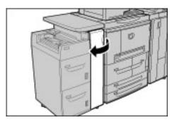
**2.** Move lever 1b to the right and turn knob 1c to the right. Remove the jammed paper.
