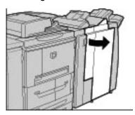
**2.** Move lever 2b, turn knob 2c to the right, and remove the jammed paper.
