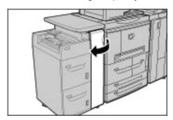
2. Move lever 1d upwards and remove the jammed paper.
