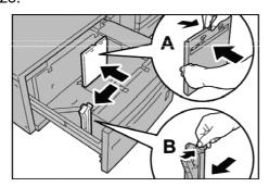
**4.** Load and align the paper stack in the lower right corner of the tray as shown below.
