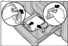
Ensure that the levers are positioned correctly.
