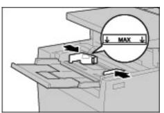
**3.** Load paper with the side to be copied or printed on facing up, and insert the paper lightly along the paper guide on the front side of the machine until it comes to a stop.
