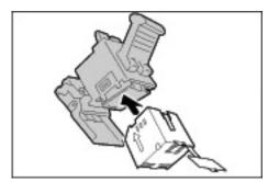
**6.** Remove the seal attached to the new staple case, as shown in the illustration.
