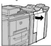
2. Pressing the lever to the right, pull out the cartridge.
