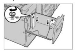
**5.** Load and align the edge of the paper against the right edge of the tray with the side to be copied or printed on facing up.
