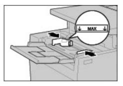
**3.** Place the paper with the side to be copied or printed facing up and the bottom side to be fed first. Insert the paper slowly to the end along the paper guide.
