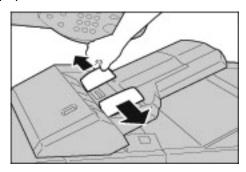
**2.** If the paper in already printed on, load the paper with the printed side facing up and with the tab side to be fed first.
