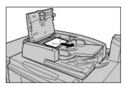
**4.** If there are instructions to turn the wheel, turn the green wheel to eject the document upward.
