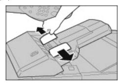
2. Load the paper, aligning to the front side of the tray.
