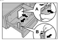
**3.** Fan the sheets before loading them into the tray. With the side to be printed on facing up, load and align the paper stack in the lower right corner of the tray as shown below.
