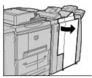
**2.** Move levers 3b and 3d to the left, and remove the jammed paper.
