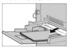
**2.** Remove the jammed paper and all paper loaded in paper Tray 5 (Bypass).
