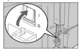
In the event of a current leakage, the breaker will automatically cut off the power circuit to prevent any leakage or fire from occurring.
