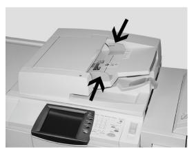
**3.** Load the document and ensure the **Confirmation** indicator lights to show that the document has been loaded correctly.
