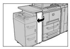
**2.** Move lever 1a to the right and turn knob 1c to the right. Remove the jammed paper.
