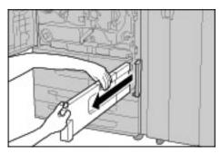
**5.** Hold the used waste toner container firmly with both hands and put it into the provided plastic bag.
