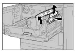
**6.** Turn the knob 2f as necessary and then remove the jammed paper.
