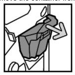
**5.** Remove the new container from the packaging. Dispose the full container in the packaging that came with the new container.
