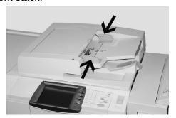
**3.** Load the document and ensure the **Confirmation** indicator lights to show that the document has been loaded correctly.
