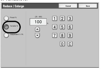
2. Specify the ratio with the numeric keypad or the **up** and **down** buttons.
