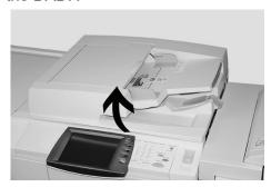
**2.** Wipe the document cover with a soft cloth moistened with water to remove any dirt and then wipe it with a soft, dry cloth.
