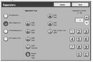
**4.** If **Blank Separator** is selected, enter the number of separators to be inserted using [s] and [t] or the numeric keypad.
