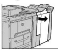
**2.** Move lever 3e, turn knob 3c to the right, and remove the jammed paper.
