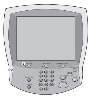
2 On the digital press control panel, press the All Services button, and then press the Web Applications button.
