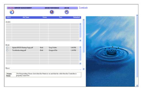
A list of jobs waiting to print at the EFI Splash RPX-iii appears, along with information about the printer and any errors that might have occurred at the printer.
