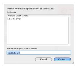
3 Select the EFI Splash RPX-iii that you want to connect to from the list of Available Splash Servers, or type the EFI Splash RPX-iii IP address in the IP address field, and then click Connect.
