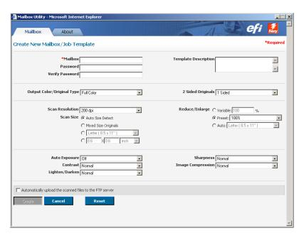
With version 1.1, you can select an option to "Automatically upload the scanned files to the FTP server". If you select this option, scans sent to this mailbox are automatically transferred to an FTP location. Fields appear that allow you to specify the details of the FTP site.
