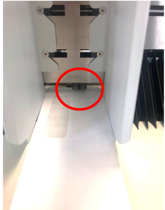
Off-centered O-ring Assembly Location - Avoids Hitting Windows on Windowed Envelopes
