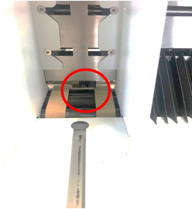
Off-centered O-ring Assembly Location - Avoids Hitting Windows on Windowed Envelopes
