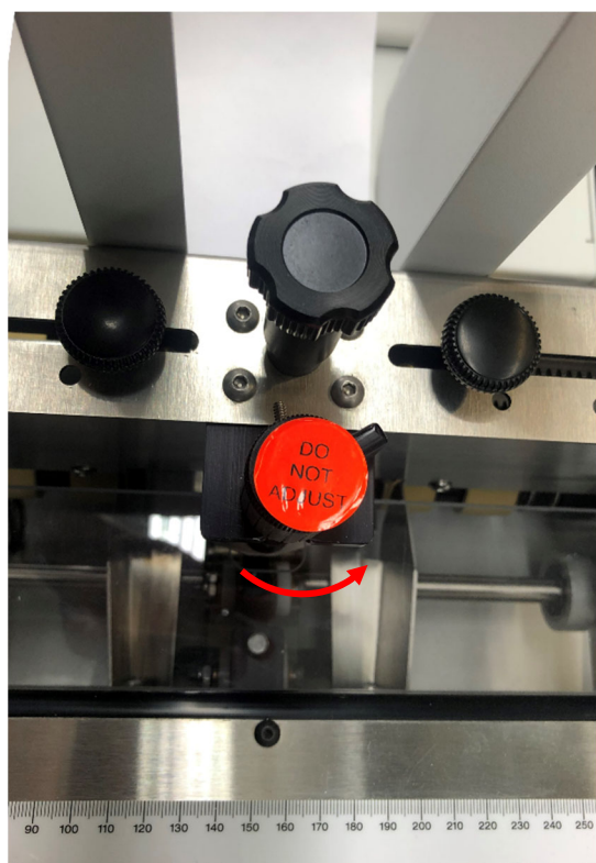
Lowering the Separator (increase friction for better separation)
