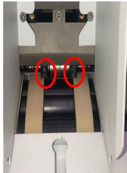
O-ring Assemblies located partially over the Belts: Ideal when using many different envelope types/substrates
