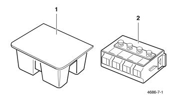
Before installing the print head, be sure to remove the packing material.
