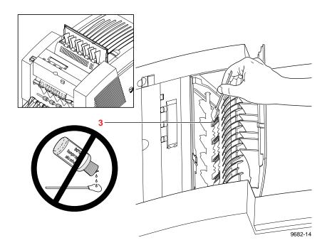
To clean the rubber exit rollers, wrap an alcohol-soaked cloth around the index finger of one hand. Press your cloth-covered finger against each roller and turn the roller several times to clean each roller individually.
