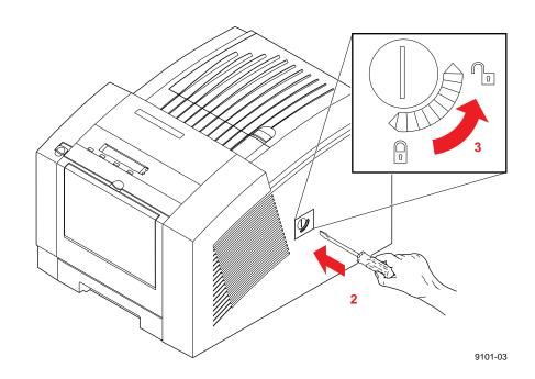
If you move or ship the printer, be sure to lock the transit Caution restraint to protect the printhead from damage. Refer to "Moving Your Printer" on page 5-39 for more information.
