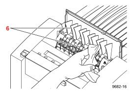
Caution To avoid damaging the print drum and exit guide, never scrape excess ink with a tool or fingernail. Use only the materials provided with the cleaning kit.
