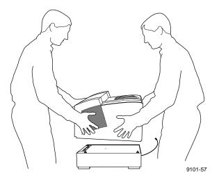
Install the Lower Paper Tray Assembly using these steps:
