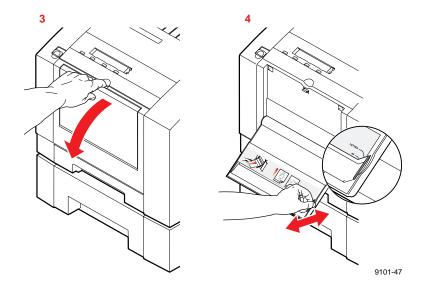
Manual feed letterhead: When you manually feed letterhead, orient the letterhead face down and feed the bottom edge first.
