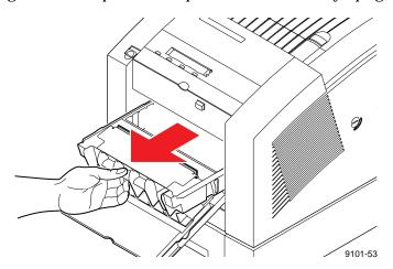
Note Once the maintenance tray has been partially used, it leaks drum fluid if tipped. Contact with the drum fluid poses no known health risk; refer to page 9-6 for more information.
