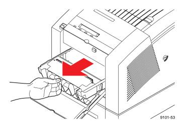
Note Once the maintenance tray has been partially used, it will leak drum fluid if tipped. Place the maintenance tray on a flat surface after removing it from the printer. Contact with the drum fluid poses no known health risk. Refer to "MSDS for silicone oil" on page 9-6 for more information.
