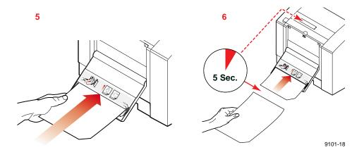
Note A jam error will occur if you feed the second sheet of media into the manual feed slot before the front panel prompts you.
