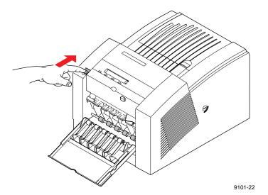
If necessary, open the exit cover using the blue release button located inside the front cover, at the top of the printer.
