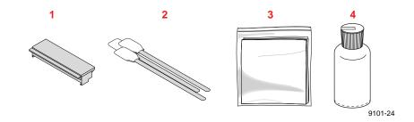
Some cleaning procedures require you to use cloth wipes or swabs saturated with isopropyl alcohol. Since shipping regulations prohibit supplying alcohol or presoaked cleaning materials with the printer, you must supply 90% pure isopropyl alcohol (available at pharmacies). You can obtain pre-soaked alcohol wipes by ordering a separate cleaning kit from Tektronix or by ordering them in packs of 10 (Tektronix order number 006-7824-01).
