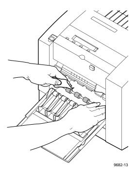
6. If the lower white plastic rollers are dirty, clean them using either the pre-packaged alcohol-soaked cloth or fold a lint-free cloth into a two-inch square and soak with alcohol.
