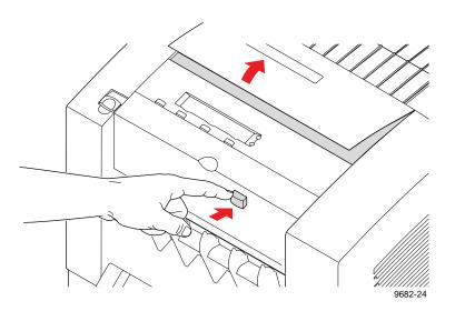
To clean excess ink particles and drum fluid from the colored exit fingers, gently wipe the top surface of each finger using a dry swab.
