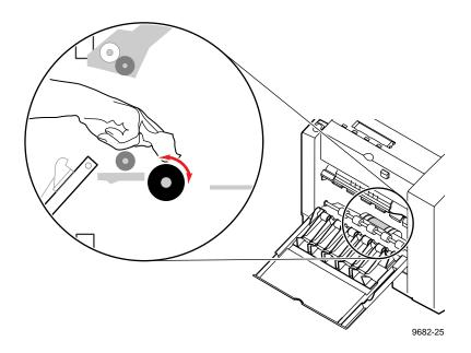
**6.** Replace the maintenance tray in the printer.
