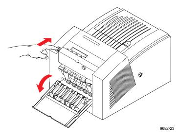
Caution Hot surfaces exist behind the upper paper-feed rollers. To avoid personal injury during cleaning procedures, do not reach in behind the paper-feed rollers.
