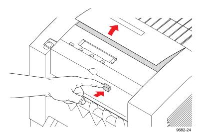
Using both hands, pull the jammed media out the top of the printer.
