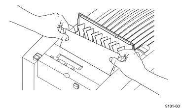
If necessary, remove the media tray to locate and clear jammed media.
