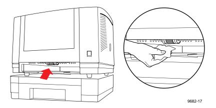
Using an alcohol-soaked cloth, scrub the bottom surface of the pick roller thoroughly.
