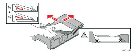
Load the second stack of paper. Make sure that the paper fits flat in the tray.
