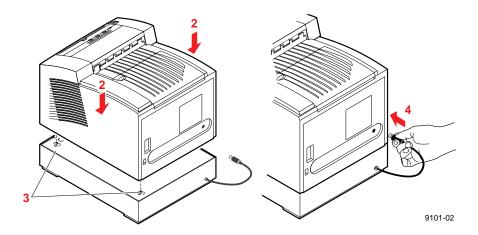
To move the printer more than a few feet, it is easier to disconnect the Lower Paper Tray Assembly and move the printer separately from the Lower Paper Tray Assembly.
