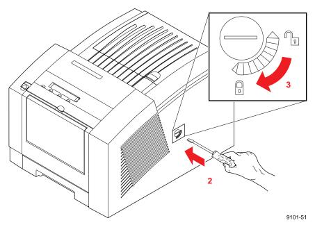
3. While pressing inward with medium pressure, turn the transit restraint slot in a *clockwise* direction to lock the printhead in position. The lock button is recessed from the side of the printer when fully engaged.
