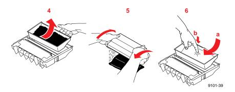
Replace the maintenance tray in the printer.
