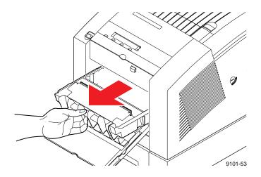
Note Once the maintenance tray has been partially used, it leaks drum fluid if tipped. Never ship a partially used maintenance tray. Contact with the drum fluid poses no known health risk. Refer to "MSDS for silicone oil" on page 9-6 for more information.
