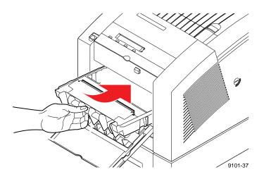
Note To prevent jams at the media tray, be sure to push the maintenance tray into the printer until both sides latch firmly into place.
