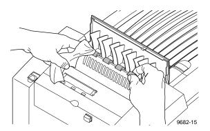
Note You may notice some staining of the exit rollers while performing the cleaning procedure. This is normal and does not indicate additional cleaning is necessary. Simply clean rollers to remove any build-up of ink.
