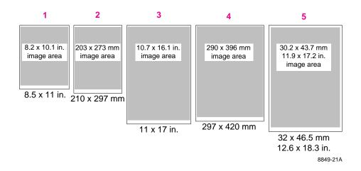
The standard tray supplied with the printer accommodates B, A3, and WB sizes. The tray for A and A4 must be ordered separately.
