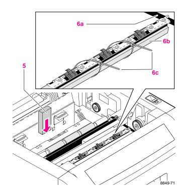
7. Place the two rubber cushions, marked L (left) and R (right), onto the metal bar on either side of the platen. Make sure that the rubber cushions are positioned with the posts *upright* (or *leaning slightly forward*) and *facing outward* as shown.
