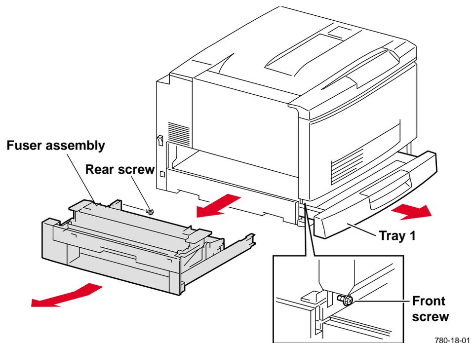
6. Tilt the end of the fuser assembly as you insert the assembly side rails into the guide wheels inside the printer. Ensure the guide wheels are inside the siderail grooves.
