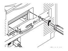
**6.** Insert the network card, or attach the lower cover plate and secure with the mounting screws.
