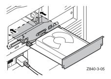
5. Secure the hard disk in place with the mounting screws and make sure that the screws are tight.
