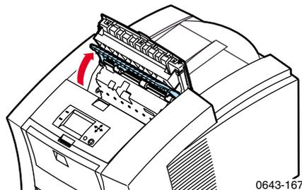
4. Handle the Rapid Release Guide carefully to avoid bending or damaging the clear plastic edge. Lift up on the blue tabs and remove the Rapid Release Guide. Do not use any sharp objects in this area of the printer.
