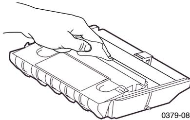
3. Reinsert the maintenance drawer into the printer.
