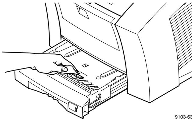
3. Inspect the separator pad for damage to the metal edge; it should be free of dents and lie flat against the rubber surface. If any damage is seen, the separator pad should be replaced (part number: 116-0838-00).
