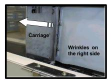
2. Check the position of the carriage. If it does not return to the home position, manually move the carriage away from the platen.
