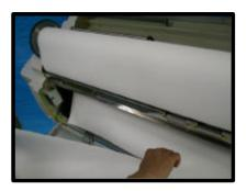
2. Carefully remove the jammed media from the cutter unit.
