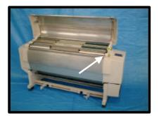
When changing media rolls, the release lever on the right side of the printer is not used and should be left in its closed position.
