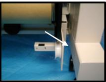
1. Adjust the position of TAKE UP ROLLER HOLDER for the roll size. Perform this action on both the left and right sides.
