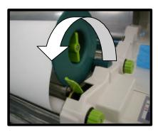
1. Open the top and front covers. Pull up the release lever to release pressure as shown in illustration to the left.
