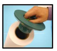
Insert an end cap into one end of the new media roll until it is firmly seated, being careful not to damage the other, exposed end of the media roll. The end cap should be snug, but not jammed on the roll for optimum use.
