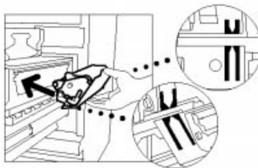
Figure 46: Aligning the new Cleaning Web
