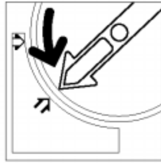
Figure 9: Rotating the Dry Ink Cartridge
