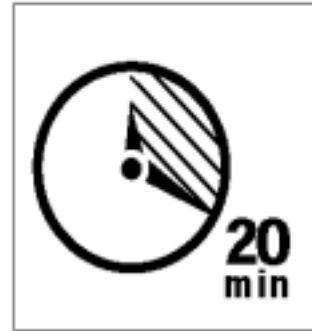
Figure 43: Allow the fuser to cool
