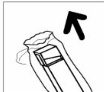
Figure 18: Removing the new Dry Ink Waste Container from the bag
