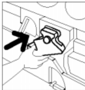
Figure 26: Inserting the new Developer Waste Container
