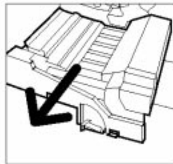
Figure 35: Pulling out the Paper Path Module
