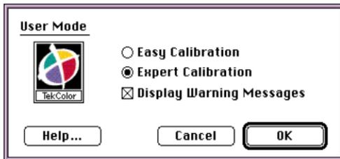
2. The **User Mode** dialog box is set to **Easy Calibration** by default at installation. Select **Expert Calibration** to activate all menus and commands.
